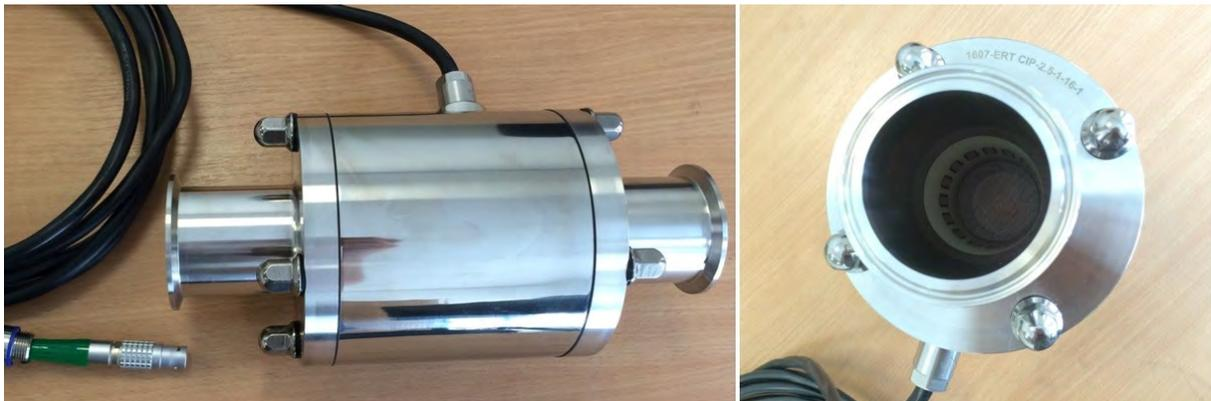
These have end coupling flanges and a cable to the processing unit. Internally they have a ring of 16 electrodes.
